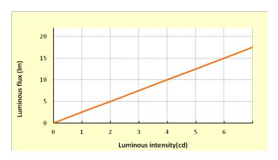
The relationship between luminous intensity (cd) and luminous flux (Lm) depends on the directionality of the product.
